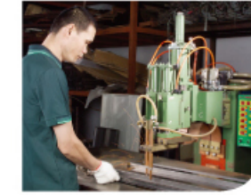
Double-welding Semi-automatic Computer Spot Welding Machine: With the welding spot exerting fast and steady pressure, the girt strip is leveled for maximum smoothness after fast welding.
