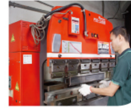
Japanese-manufactured computer-controlled Bending Machine: Produces smooth and accurate curves.
