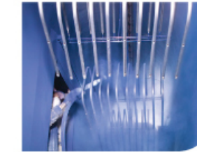
Powder Bake Coating: shown in automatically controlled tunnel
